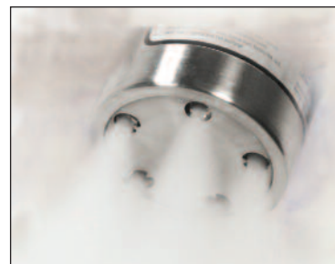
Aerosol generator discharge
